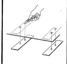
Pull up the carpet, peel off the protective paper of tape (a) to expose the adhesive on the bottom of the plates (2) and place the unit in the desired installation position so that the plates adhere to the surface.
