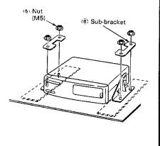
Installation method 1 is a simple installation method. If the sound skips when CDs are played, reinstall the unit using installation method 2 (see the next page.)
