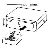
To remove the disc magazine, open the door and then press the EJECT switch,
