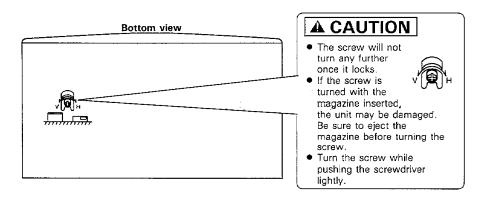
Vertical installation (Turn the screw 180° to the left.)
