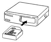
Insert the disc magazine into the unit.
