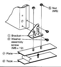
2 Pull up the carpet, peel off the protective paper to expose the adhesive on the bottom of the plates ② and place the unit in the desired installation position so that the plates adhere to the surface.
