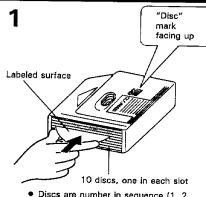
Discs are number in sequence (1, 2, 3...) from the bottom slot up, insert discs into the magazine with their labeled sides facing up.
