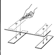
With the carpet in place, use the 4 nuts (M5) (6) to secure the changer in the installation position.
