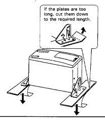
3 Cut the carpet at the points where the plate ② bolts protrude.
