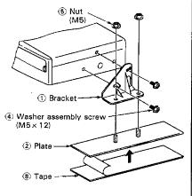
3 Cut the carpet at the points where the plate ② bolts protrude.
