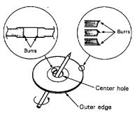
Before using a new disc, be sure to check for burrs around the edges of the disc's center hole and outer circumference (see diagram at left). If burrs are present, use a ballpoint pen or similar instrument to remove them. If a disc is used with burrs still attached, the disc may not fit properly in the player or disc magazine, or the sound may tend to skip during playback.
